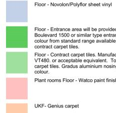
Floor - Contract carpet tiles. Manufacturer: CFS Illusion or CFS VT480. or acceptable equivalent. To staircases provide contract carpet tiles. Gradus aluminium nosing's to all treads in contrasting colour.
